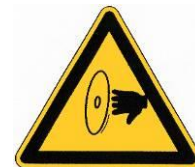
Danger: risk of cut
