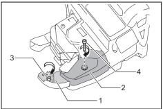
1. Wire guide B 2. Contact plate cover 3. Bolt A
