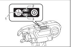
Mode switching button 2. Single actuation mode
