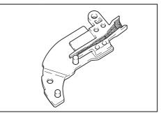
**5.** Remove cutter A, cutter B, top plate, and link arm A from arm plate A. Then, clean them.
