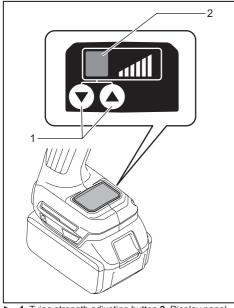
Tying strength adjusting button 2. Display panel
