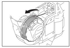
**9.** Release the lock lever. The release lever returns, and the wire is held by the left and right gears.
