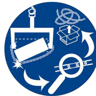
If the load falls into the load securing chain, the chain must be checked professionally and replaced if necessary. Do not continue to use damaged load-securing chains!
