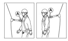
ATTENTION: Every time before using the equipment protecting against falls from height that employs the AC010 one needs to check if all the components are properly interconnected to one another and cooperate smoothly, as well as if they are compliant with compulsory standards:
