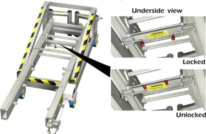
**2.** Lock foot operated castor brakes before raising mast.
