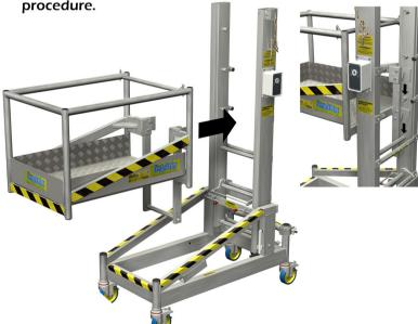
7. Locate top half of quard rail assembly onto bottom half platform quard rail assembly. This is a two person procedure.
