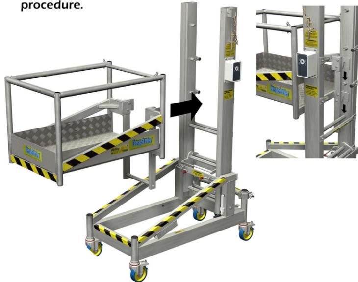
7. Locate top half of guard rail assembly onto bottom half platform guard rail assembly. This is a two person procedure.
