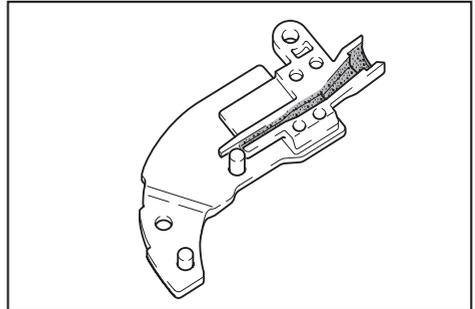
5. Remove cutter A, cutter B, top plate, and link arm A from arm plate A. Then, clean them.
