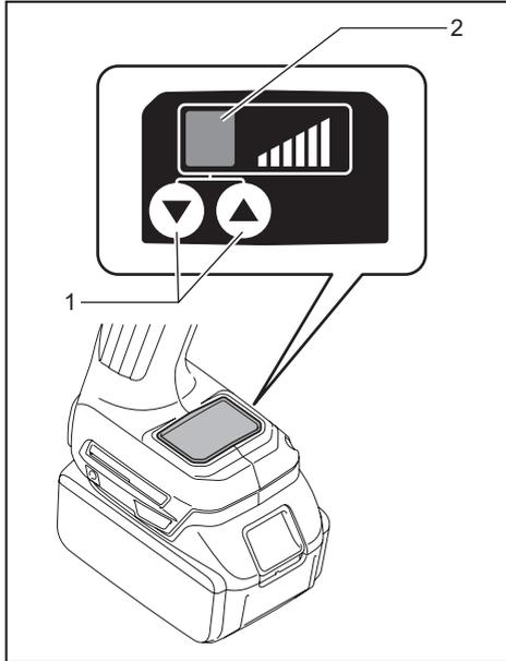
► 1. Tying strength adjusting button 2. Display panel
