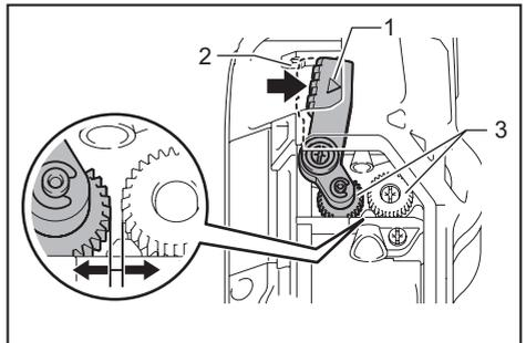
► 1. Release lever 2. Lock lever 3. Feed gears
