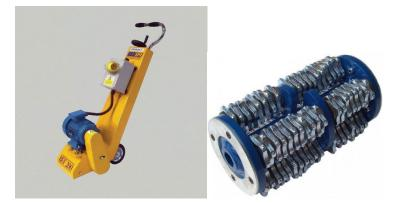
This electric floor planer is for use on concrete floor slabs to smooth the surface, flatten uneven surfaces or remove sealants etc. Cleaning and Texturing concrete and asphalt. Removal of paint, rust, grease, ice deposits, line markings, and concrete laitance. Also removal of roof chippings. Dust Extraction option available
