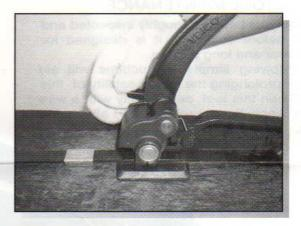
Press the handle pawl down so that the handle can be released. Place the seal open side down over both straps in front of the tool.
