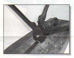
Open the sealer fully open position, put the sealer on the top of the seal, press the sealer handle together to fully crimp the seal, then remove the sealer.
