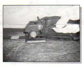
Compress down the handle to lift the feedwheel. Slide the tool away from the strapping material. Cut excess strap with a steel strapping cutter.
