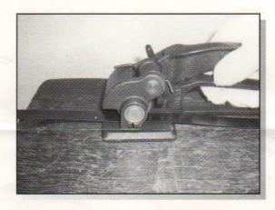
Compress the handle to lift support frame.
