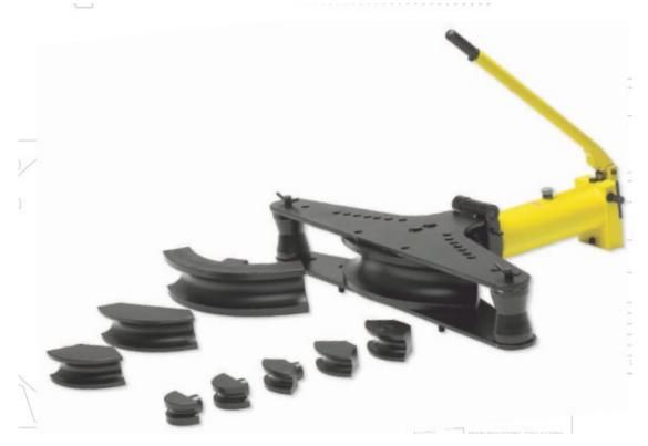
Manually operated Hydraulic Pipe Bender having a hinged frame design incorporates the benefits of high performance combined with low weight, making it a professional portable tool. Bending sizes from 3/8" up to 2" designed for precision cold bending of standard gas pipe and black pipe up to 2"
