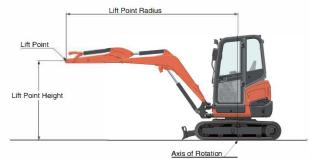
\* Working ranges are with Kubota standard bucket, without quick coupler
