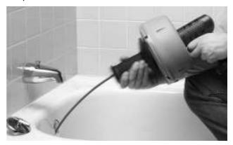
Figure 5 - Pull Hand Grip Rearward To Engage Clutch
