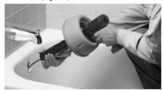
Figure 8 – Keep Distance Between Drain Opening and Nose of Drain Gun to 6" or Less
