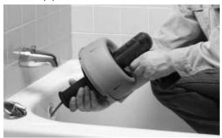
Figure 6 - Push Cable Down Drain Line
