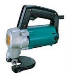
A Powerful hand held tool for heavy cutting of mild and stainless steel, Metal Shear for straight and curved cuts with a radius of 50 mm, cuts a clean-edged strip from the middle. A high cutting capacity of 3.2 mm for mild steel, and 2.5mm in Stainless Steel.
