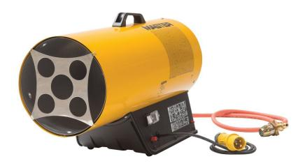
Space heater is a portable unit, that is powered by propane gas and requires a mains power supply. It produces direct fired heat and is fan assisted in order to heat small and large spaces quickly.
