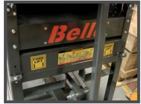
FORKLIFT POINTS FOR SAFE ON-SITE TRANSPORTATION
