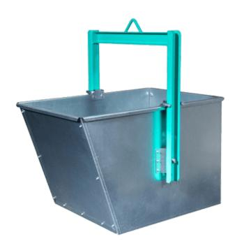
The Muck Tipping Bucket with fold-down hanger and safety locks. When the safety locks are opened by hand the tub empties automatically in response to the centre of gravity of the hanger.
