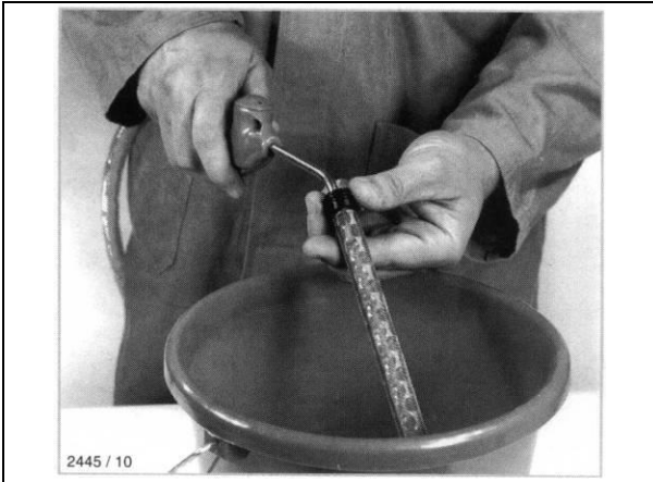
Use an air line to blow out oil filter dirt from the inside outwards.
