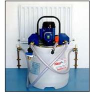
power flushing is commenced. This is likely to be the least effective method due to the restrictive effect that valves (particularly thermostatic) may have on the flow rate.
