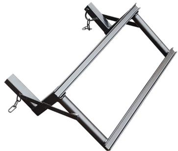
**From a parapet or window**, the first rubbish chute bracket is connected to the chain from the window. Always ensure the spreader bar is fitted to ensure an even distribution of weight, and the parapet is capable of taking the strain you will put on it.
