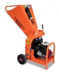
Being both robust and hand portable, the 13/75 is very easy to manoeuvre into confined spaces. Handles material up to 75mm (3") with ease. This is the most favoured by professionals working in confined spaces.
