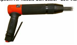
This air driven needle gun does a thorough job of exposing reinforcing steel, removing residues from formwork, cleaning metal and moulded parts, roughing stone and concrete. Always use an In Line Oil Lubricator and Moisture Separator with these tools. Attach the In Line Oiler Lubricator as close to the tool as practical.
