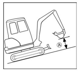
• When driving on gradients, let the bucket slide over the ground if the terrain allows it.
