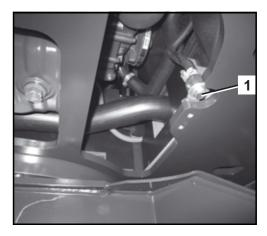
• Remove the coolant expansion reservoir (1) and drain it, cleaning it if necessary. Refit the reservoir.
