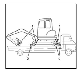
• Lock the excavator after hoisting.
