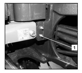
• Operate the excavator and swivel the swivel frame by 90° several times. After greasing, swivel the swivel frame 360° several times to distribute the grease evenly.
