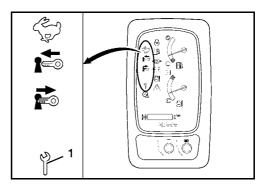
If the maintenance interval indicator has to be replaced because of a defect, the meter is set back to "0". Ask your KUBOTA dealer about this.
