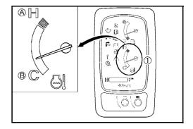
If the coolant temperature is too high, cool down the engine by changing into idle. The display message as in the figure on the right appears.
