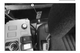
1) Code #: R2491-5796-0 Attachment point for lifting gear.
