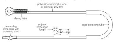
Using the work positioning device PROT-2 in connection with connectors must be compatibile with their instructions and obligatory standard EN 362.
